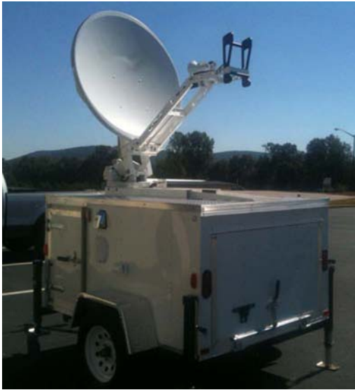
The PathFinder Transportable SatCom System Platform as shown above is outfitted with a 1.2 meter auto-acquisition satellite antenna and a dual WiFi broadband system.
